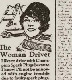
Champion is the better spark plug because it has an exclusive sillimanite insulator specially treated to withstand the much higher temperatures of the modern high-compression engine. Also a new patented solid copper gasket-scal thatremains absolutely gas-tight under high compression. Special analysis electrodes which assure a fixed spark-gap under all driving conditions. HAMPION
